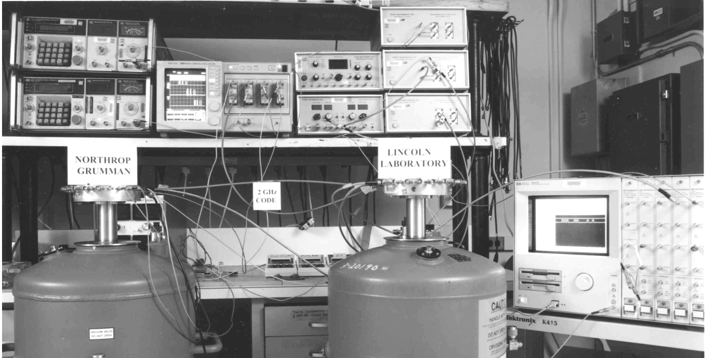
Fig. 4. Josephson digital circuits in separate cryostats transferred data through more than 3 meters of cable at 2 Gbps without using semiconductor amplifiers.
